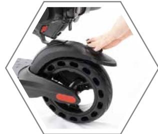
Align the latch on the mudguard with the attachment point and connect
