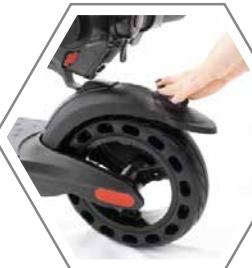
Release the rod by applying pressure to the mudguard
