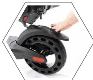
Release the rod by applying pressure to the mudguard
